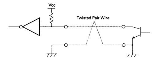
All the output signals are pulled up by  $50K\Omega$ .
